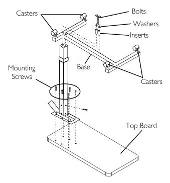
FIGURE I Assembling the Overbed Table - Model 6417
